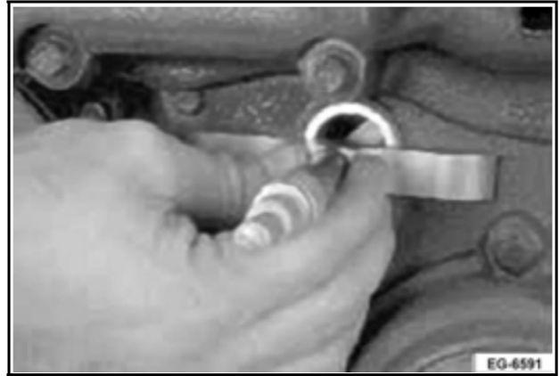
Figure 382 Measuring the Sensor Air Gap
