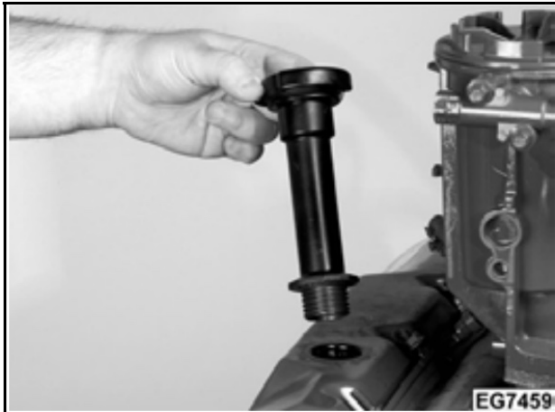
Figure 184 Installing the Oil Filler Standpipe
