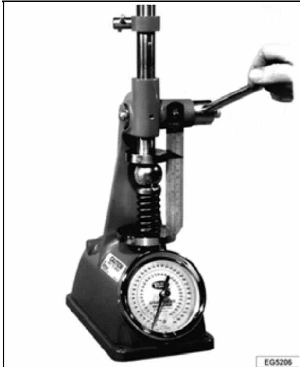
Figure 140 Testing Operation of Valve Rotators
