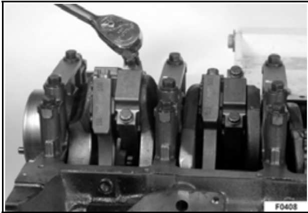
Figure 269 Removing the Connecting Rod Cap
