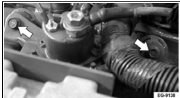
Figure 360 ECM Support Assembly Upper Mounting Bolts
