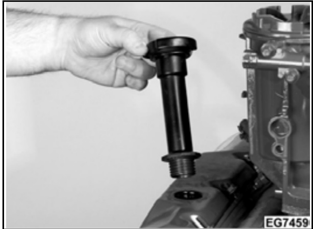
Figure 101 Removing the Oil Filler Standpipe
