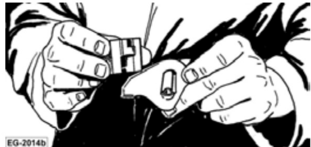
Figure 165 Installing the Valve Lever Post
