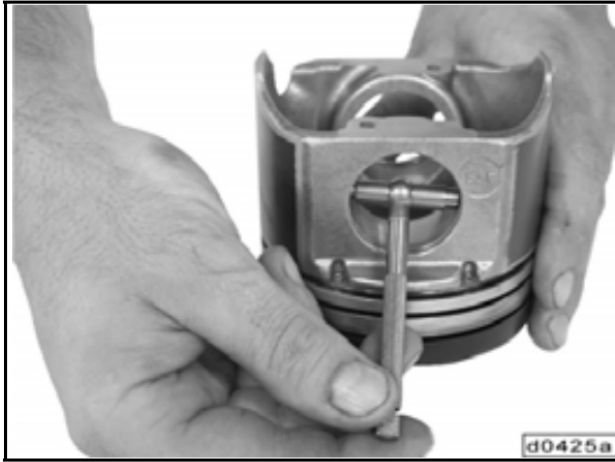
Figure 285 Measuring Piston Pin Bore Inside Diameter
