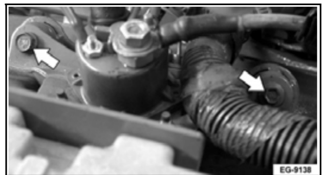
Figure 364 ECM Support Assembly Upper Mounting Bolts
