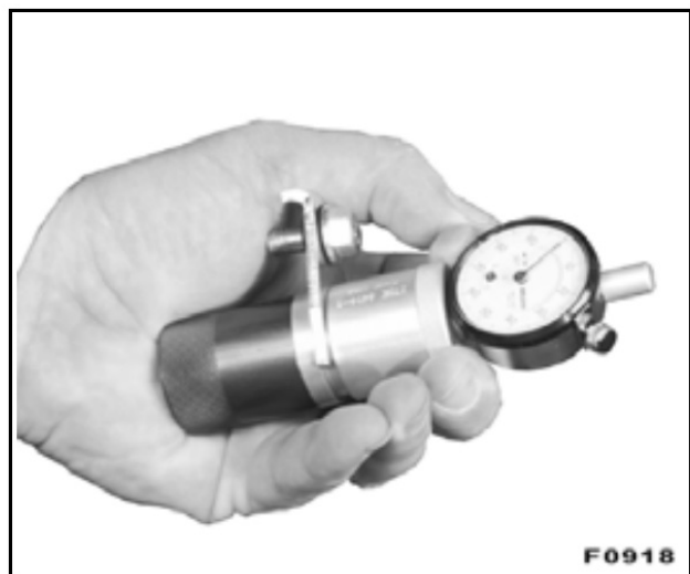
Figure 381 Camshaft Sensor Air Gap Tool In CMP Sensor
