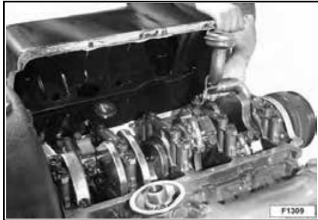
Figure 192 Removing the Oil Pan From the Crankcase
