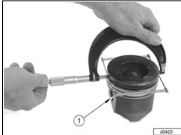
Figure 278 Measuring Top Compression Ring Groove
